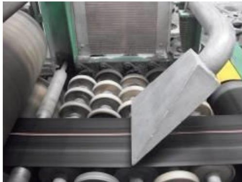
**Fig. 5: Production of outer rubber sheets for motorcycle tires**
