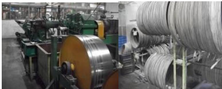
**Fig. 6: Production of wire frame for motorcycle tires**
