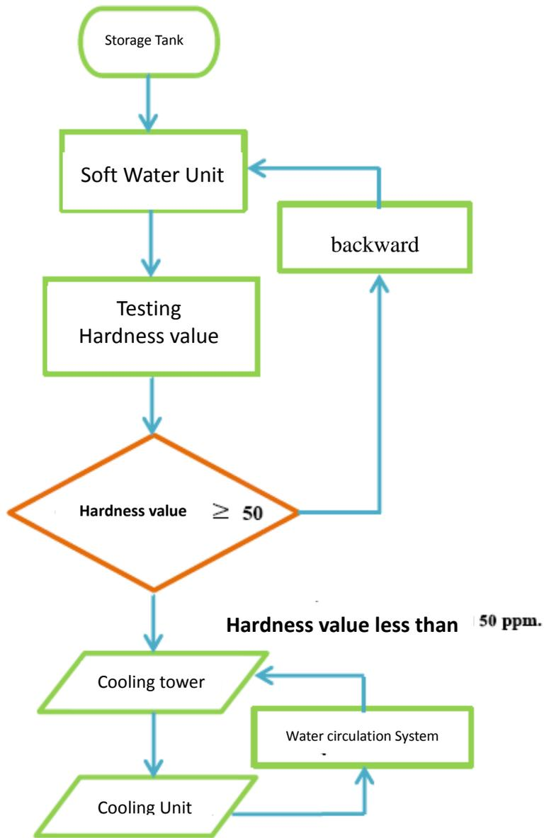
Fig. 1 The process produces soft water
