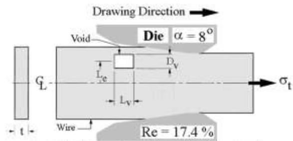
Fig. 1 Model of copper shaped-wire contain a void used in this analysis
