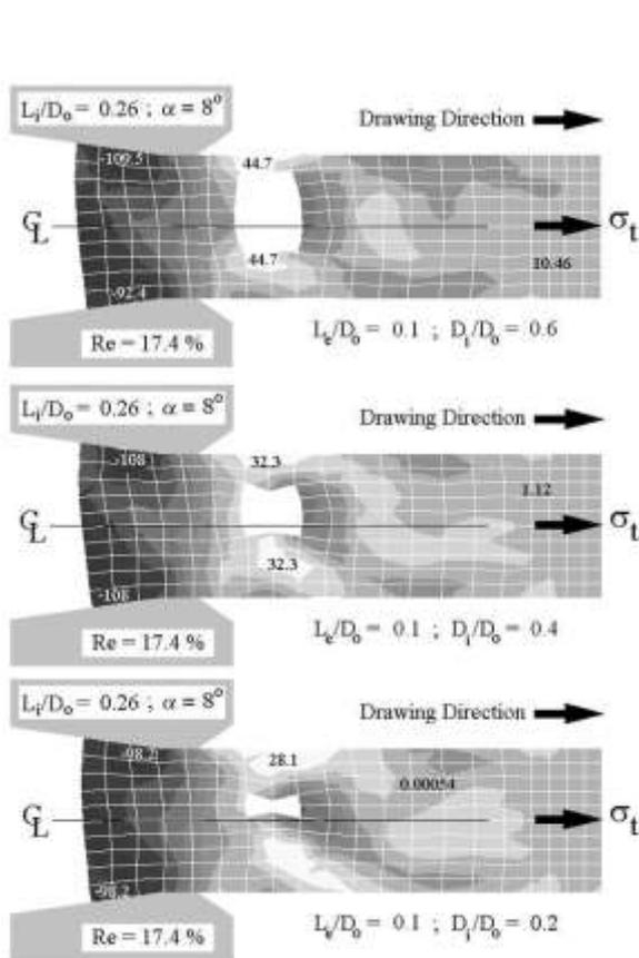
**Fig. 3** The deformation and mean normal stress distributions of copper wires contain a constant eccentric length various size void
