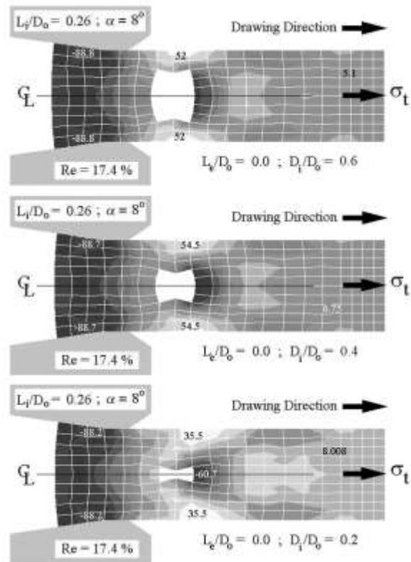
**Fig. 4** The deformation and mean normal stress distributions of copper wires contain a central various size void
