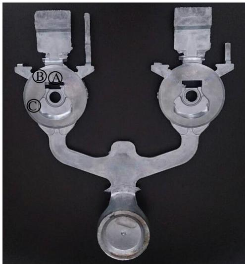
**Figure 2.** Motorcycle fuel caps of an original HPDC part.
