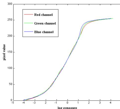
Fig. 3. The response curve of a Nikon D70s camera
